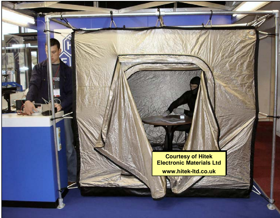
Figure 4BV Example of a shielded tent made from metallised fabrics
